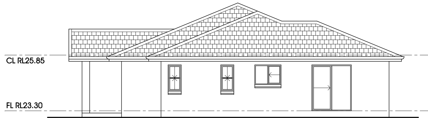
south west elevation
